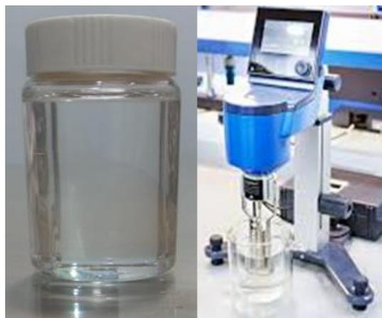
**Figure 2.** The dynamic (absolute) viscosity of the nanoemulsion was determined using a Rotary Myr VR 3000 digital viscometer.
